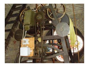
The movement was electrified at an unknown point in history. The weights and several other components were removed as part of the conversion; the governors are still in the tower next to the clock. The clock is not currently running, but members of the congregation still climb the steep stairs to the tower on Sundays to ring the bells
